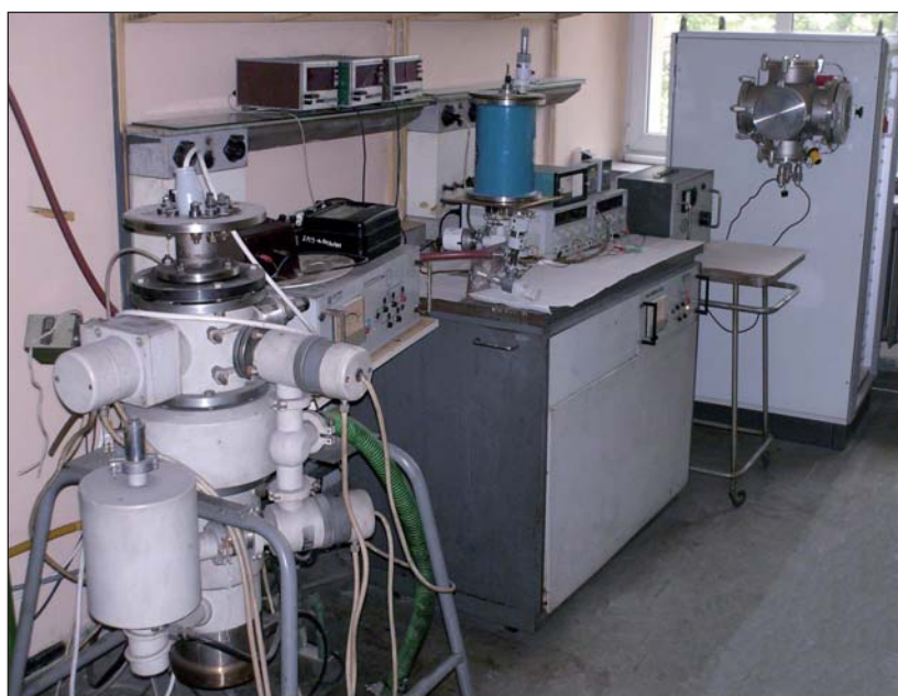
Fig. 1. Technological setup for producing polymer layered structures (J. Weszka)
