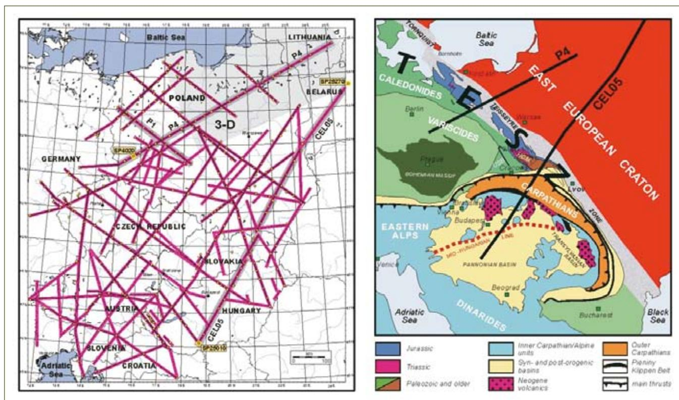
Fig. 2. Location of seismic profiles in the international modern seismic experiments POLONAISE'97, CELEBRATION 2000, ALP 2002, SUDETES 2003 (left side). White circles – shot points for generation of seismic waves; P1, P4 and CEL05 – main profiles for seismic experiments POLONAISE'97 and CELEBRATION 2000. Total length of all profiles is about 20,000 km. Basic seismic profiles for geodynamics of the Central Europe P4 and CEL05 (right side). TESZ – Trans-European Suture Zone.
