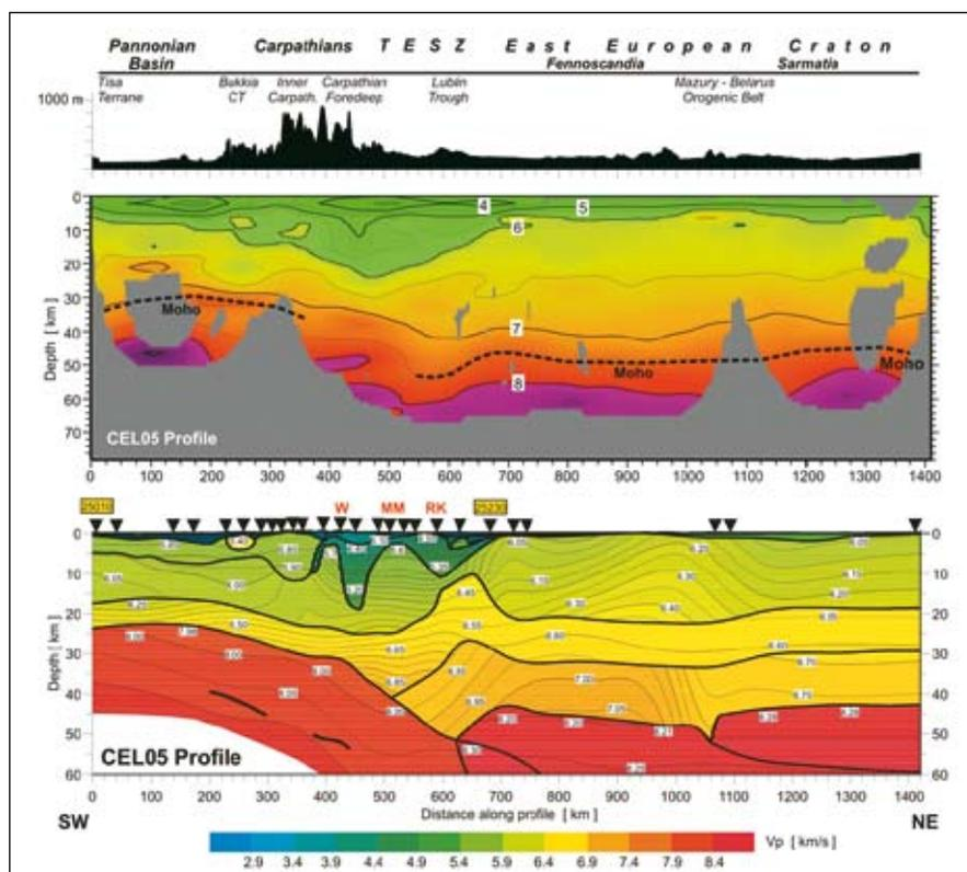
Fig. 4. Two dimensional seismic model of the Earth's crust for CELEBRATION 2000 profile CEL05 (location in Fig. 2) obtained by tomographic inversion of P wave first arrival travel times (upper Figure) and by ray-tracing modeling (bottom Figure).
