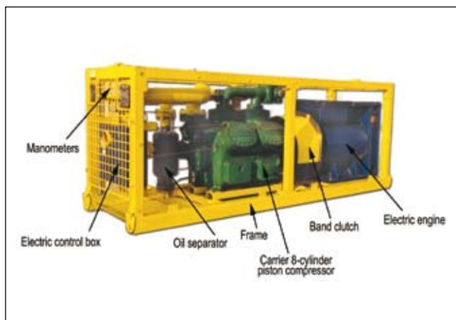
The indirect-use TS-450 refrigeration machine is designed for cooling air in underground pits, tunnels, etc. It is comprised of the following:
